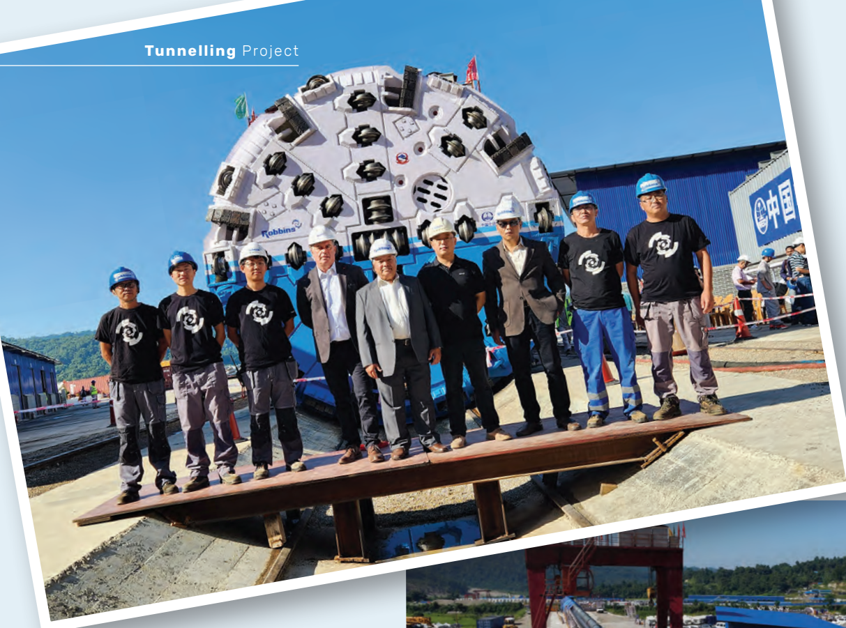
LEFT: The Robbins double shield is suitable for ground conditions including granitic rock with sections of squeezing ground and fault zones with potential water inflows.
