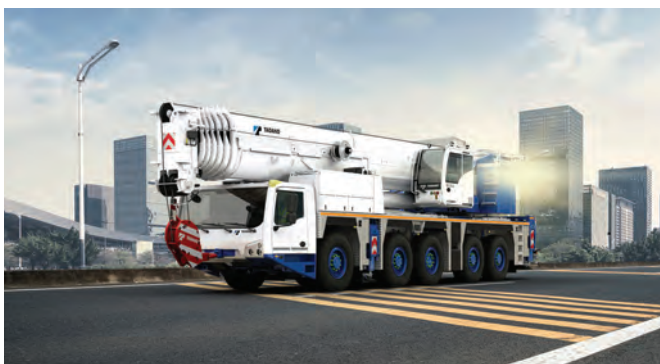
TOP, ABOVE AND RIGHT: The AC 5.250-2 all-terrain crane has a main boom length of 70 m, which can be extended by 42 m with a HAV main boom extension, allowing it to reach a system length of 112 m.
