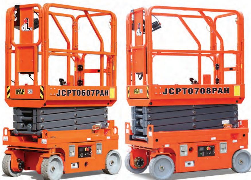
The new JCPT0607PAH (left) and JCPT0708PAH mini scissor lifts with large wheels are part of Dingli's oil-free & all-electric series.
