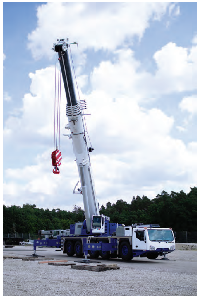
TOP, ABOVE AND RIGHT: The AC 5.250-2 all-terrain crane has a main boom length of 70 m, which can be extended by 42 m with a HAV main boom extension, allowing it to reach a system length of 112 m.
