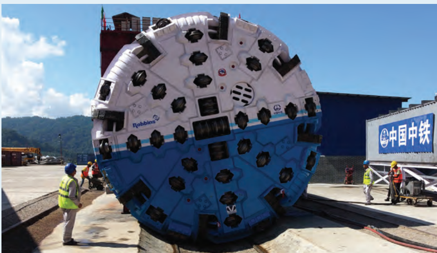
Since its launch in October 2022, the double shield TBM has bored over 500 m, with a best week of 224.6 m and a best day of 36.6 m.
