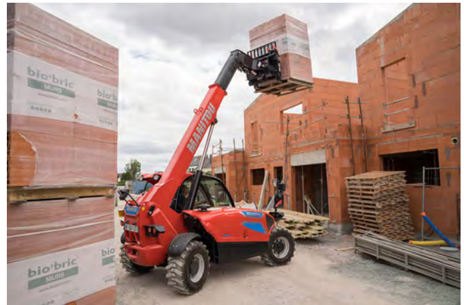
RIGHT AND BELOW: The MT 625e electric compact telehandler comes with a 25 or 33 kWh lithium-ion battery. The machine features a capacity of 2.5 t and a height of 6 m.
