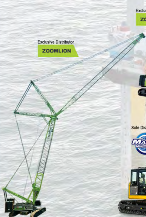
Crawler Crane with luffing jib
