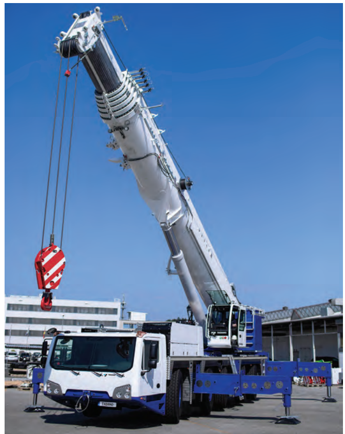
TOP AND ABOVE: The AC 5.250-2 can be used as a taxi crane without a support vehicle while remaining within the legal axle load limit of 12 t.
