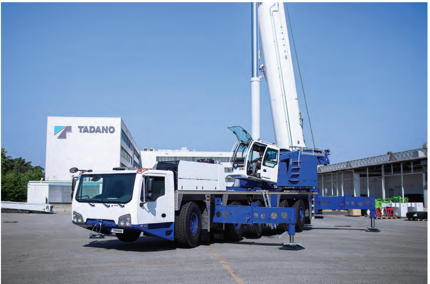
TOP, ABOVE AND BELOW: The AC 5.250-2 can pick up its total counterweight of 80 t in three lifts: 46.6 t with a full 360° radius of up to 6.2 m followed by two lifts of 15.2 t, with each split into 10 and 5.2 t for mounting on the right and left of the base package.
